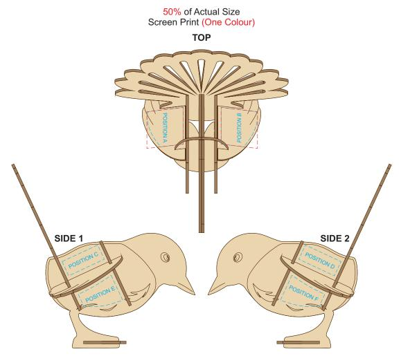
Up to a 2mm tolerance is expected for alignment of the printed artwork against the engraved lines. Slight inconsistencies are to be considered acceptable if the artwork is printed over an engraved line.
